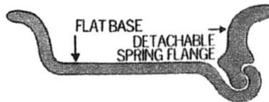
Figure 8 The principle of the 'straight sided' rim
